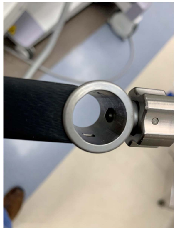
Figure 7. Demonstration of the depressable ball bearing that engages with the dimple to allow for in-line screw trajectory through the rod.
