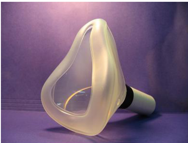
Figure 3 Picture of the oronasal mask used to measure nasal, mouth, and nasal plus mouth resistances. This mask was attached to the APD through a regular cardboard mouthpiece that fits over the pneumotach entrance.
