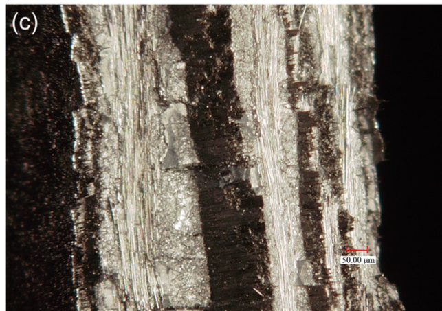
Figure 5. (a) The transverse cracks in the 90° plies; (b) the mode 3 and mode 5 cracks in 0° plies; and (c) the fracture surface of fatigue failure specimen at room temperature observed under optical microscope.
