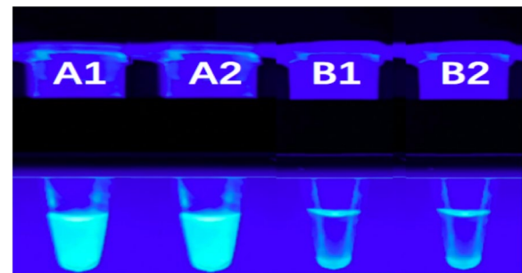
Fig. 3 Visual detection of LAMP amplification products in genomic DNA isolated from V. vulnificus . The figure indicates fluorescence for genomic DNA of V. vulnificus . (A1) V. vulnificus . (A2) V. vulnificus . (B1) Blank control. (B2) Blank control
