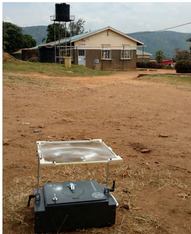
FIGURE 2. KS-Detect System in Solar Heating Mode deployed outside of a rural clinic near Kampala, Uganda.
