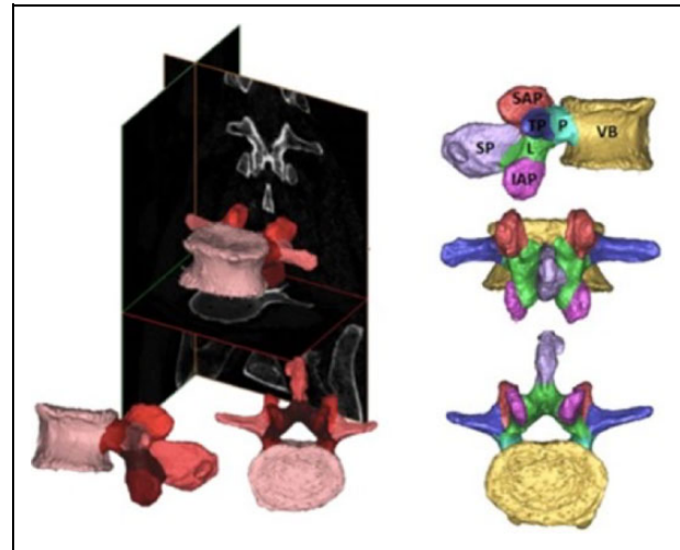
Figure 1. Images depicting the data collection process, including the conversion of computed tomography (CT) scans to engineering solid models. The 2-dimensional images (left) are segmented from a series of CT images to define volumes. Each vertebra was divided into 7 regions (right) followed by further segmentation of cancellous and cortical bone within each anatomic volume. SAP, superior articular process; IAP, inferior articular process; L, lamina; P, pedicle; SP, spinous process; TP, transverse process; VB, vertebral body.
