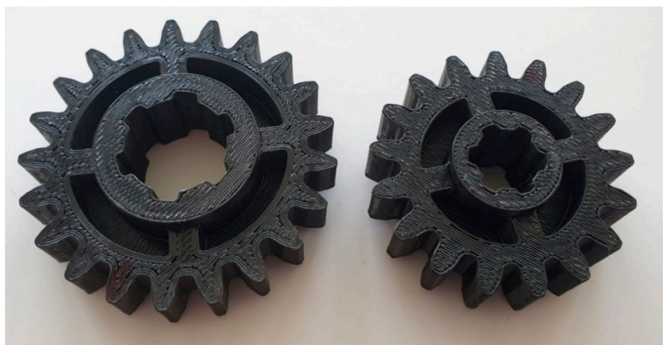
Figure 2. Gears manufactured using the FDM technique from ULTEM 9085.
