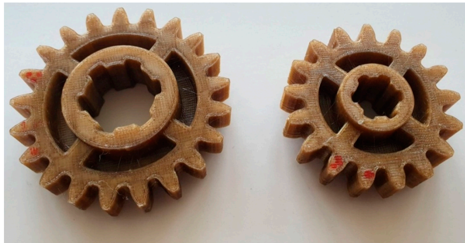
Figure 3. Gears manufactured using the FFF technique from PEEK.
