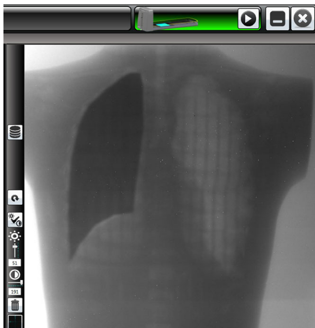
FIG. 10. Screen capture of imaging subsystem user interface showing an AP image of the end-to-end phantom with the right lung blocked and left lung unblocked.
