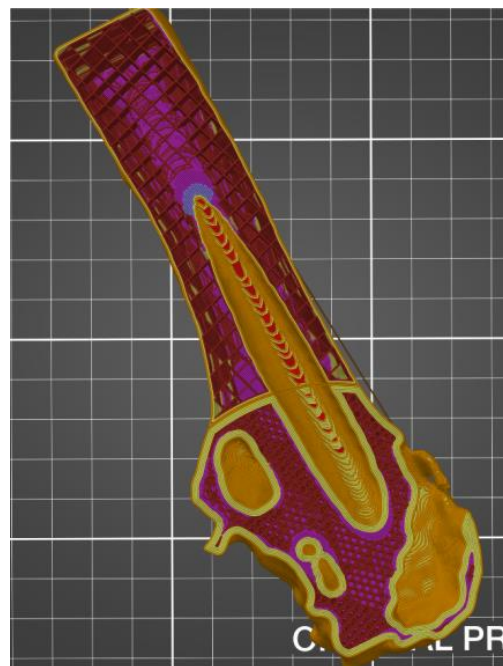
Figure 11. View of the anatomical model of the part of the femoral bone in the working space of the PrusaSlicer silver with the added modifier rendering it possible to change selected parameters.
