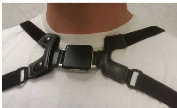
Figure 1. Image of the harness and IMU (APDM Opal Monitor) noting location of sensor package at the top of the sternum.
