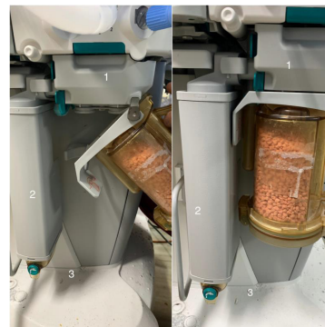
Figure 1: Canister on the machine with EZchange option. Note: 1: EZchange Canister manifold; 2: condenser; 3: drain button.
