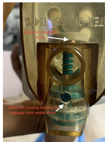
Figure 2: Leak site in the condenser assembly.
