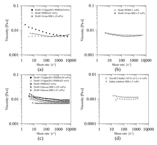
**Figure 5.** Steady shear viscosity curves as a function of the shear rate obtained by: (**a**) Calejo et al. [54], (**b**) Carvalho et al. [49], (**c**) Pinho et al. [55], and (**d**) Muñoz-Sánchez et al. [44].
