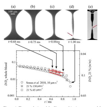
**Figure 9.** Time evolution of the filament thinning process of the particulate analogue fluid of 21 wt% PDMS microparticles suspension in an aqueous solution of 4 wt% SDS, in comparison with the blood (circles) [52]. The red lines point out the linear fit to obtain the extensional relaxation time  $\lambda$ . Reproduced from Ref. [52] with permission from The Royal Society of Chemistry.
