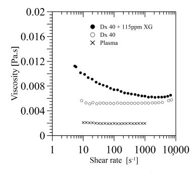
**Figure 8.** Steady shear viscosity curves as a function of the shear rate obtained by Brust et al. [24] for blood plasma, and Pinho et al. [55] for Dx40 and Dx40+115 ppmXG.
