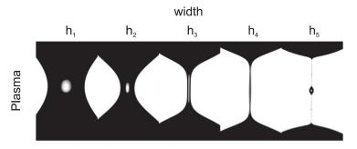
Figure 10. Images of the capillary break extensional experiment [24].
