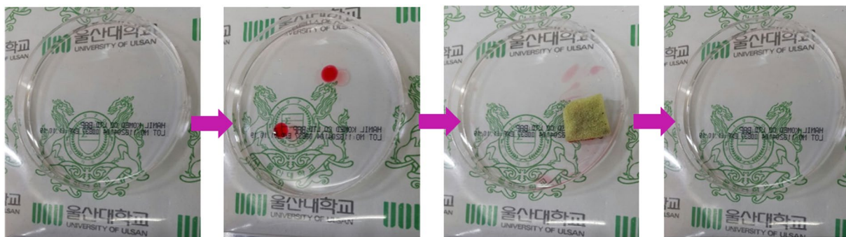
Figure 7. Photographs of using PU@ZnO@Fe 3 O 4 @SA to remove floating oil.
