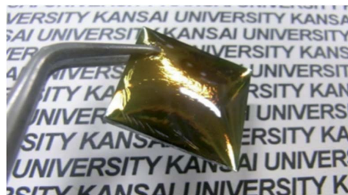
Fig. 1 Photograph of the solidified product that was prepared by dropping the concentrated solution on a square Si(100) substrate, followed by drying at 120 °C.
