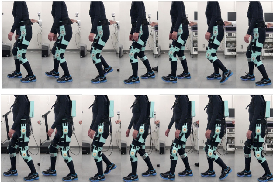
Fig. 4 Sequential photographs of a SCD patient without and with gait support during walking tests. Top panels show a patient's gait before being attached to the power units at each joint. When patients walk without gait support from the curara system, they continue to wear the joint supports molded from deformable plastic. These structures do not disturb the patient's natural gait because they are completely disconnected from the power unit, so there is no assistive torque. This condition is thus equivalent to not wearing the assistive robot. Bottom panels show the patient's gait while walked after being outfitted with the curara system, which provides gait support
