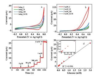
**Figure 6.** CV of alkaline *o*-phthalatocuprates in (**a**) background electrolytes and (**b**) in the presence of 3 mM of D-glucose. (**c**) Chronoamperogram of **I**/GCE recorded under potentiostatic conditions 0.55 V and (**d**) calibration curve for I obtained from CA data (Faraday current vs. [D-glucose]).
