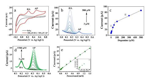
**Figure 7.** (**a**) CV of disodium di-*o*-phthalatocuprate–based electrode in background electrolyte and in presence of DA and AP; (**b**) DPVs of I/GCE recorded in mixture containing 50  $\mu$ M AP with different concentrations of DA; (**d**) 20  $\mu$ M DA with different concentrations of AP; the linear relationship between peak currents and the concentrations of (**c**) DA and (**e**)AP.
