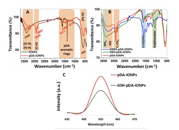
**Figure 3.** (**A**,**B**) Fourier transform infrared (FTIR) spectra showing the successful conjugation of pDA and GSSG molecules on IONPs; and (**C**) fluorescence spectra of pDA-IONPs and GSH-pDA-IONPs with  $\lambda_{\text{excitation}} = 400 \text{ nm}$ ,  $\lambda_{\text{emission}} = 450 \text{ nm}$ .
