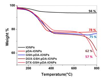
**Figure 8.** Thermogravimetric analysis (TGA) curves showing the sequential grafting of different organic molecules on the surface of IONPs.
