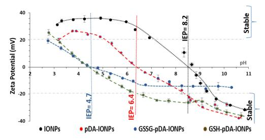
**Figure 2.** Zeta potential vs pH curves showing the isoelectric point of differently functionalized nanoparticles in  $10^{-2}$  M NaCl.
