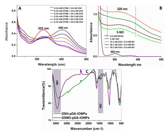
**Figure 6.** UV-visible spectra showing (**A**) the reduction of GSSG into GSH-pDA-IONPs; (**B**) S-nitrosation of GSH-pDA-IONPs; and (**C**) FTIR spectra of GSNO-pDA-IONPs and GSH-pDA-IONPs.
