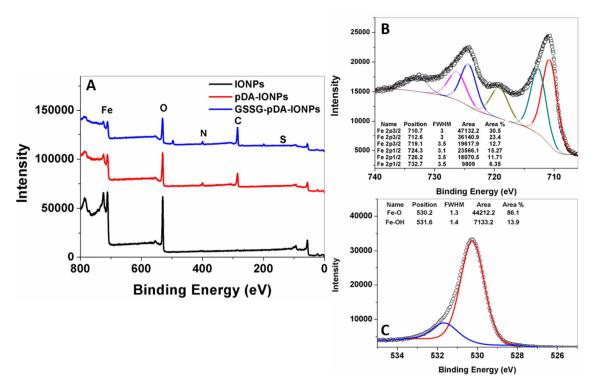
and 531.6 eV, which are attributed to the binding energies of Fe–O–Fe and Fe–OH bonds as shown in Figure 4C [43].
