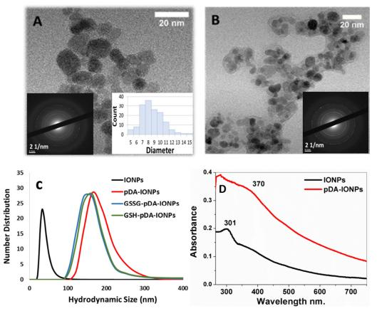
**Figure 1.** Transmission electronic microscope (TEM) images of (**A**) bare IONPs; and (**B**) pDA-coated IONPs (inset selected area (electron) diffraction (SAED) patterns and size distribution); (**C**) Dynamic light scattering (DLS) measurements showing the hydrodynamic diameter at pH = 5.0-6.0 and in  $10^{-2}$  M NaCl; and (**D**) UV-vis spectra of the synthesized nanoparticles.
