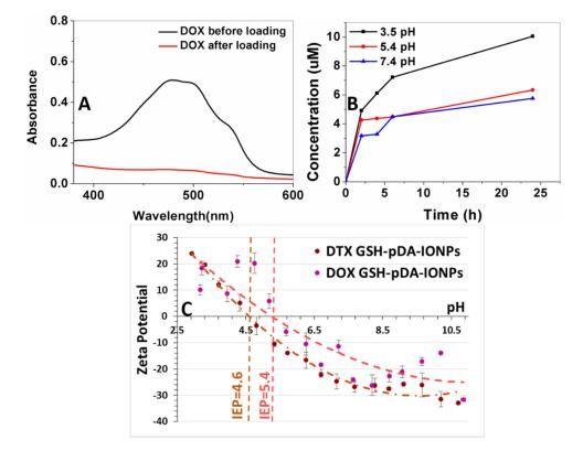
**Figure 7.** UV-vis absorbance spectra showing (**A**) doxorubicin loading on GSH-pDA-IONPs; (**B**) doxorubicin release at different pH in PBS (10 mM); and (**C**) zeta potential vs. pH curves of DOX- and DTX-drug loaded nanoparticles.
