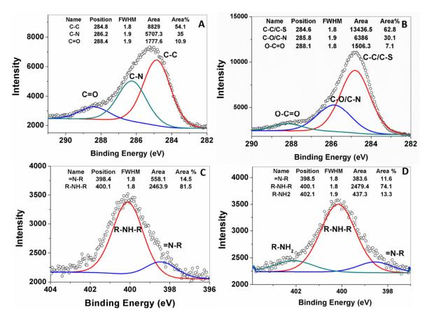
**Figure 5.** Fitted spectra of C (1s) for (**A**) pDA-IONPs; (**B**) GSSG functionalized pDA-IONPs; and of N (1s) for (**C**) pDA-IONPs; (**D**) GSSG functionalized pDA-IONPs.
