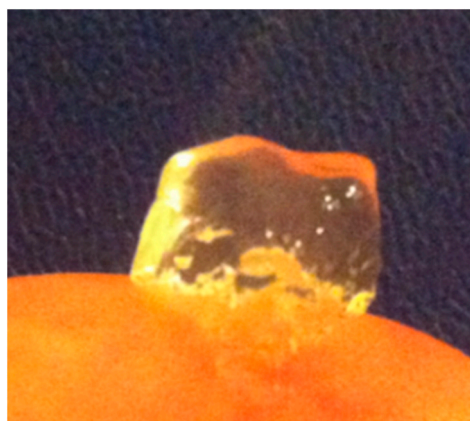
Figure 12. Photo of hydrogel on the base of N-succinyl chitosan and hyaluronic acid dialdehyde, containing MMC.
