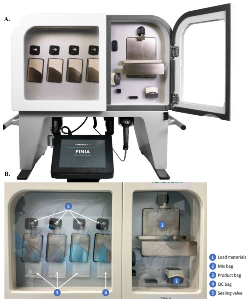
Figure 3. The Finia Fill and Finish System. A. The Finia system with general user interface and barcode scanner underneath the equipment manifold. B. Finia system setup with FINIA 50 tubing set.
