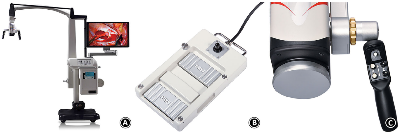
Fig. 1 (A) Kestrel View II exoscope applies fully balanced vibration absorbing system from astronomical telescope; (B) a foot switch helps for fine-tuning of focal length and changing where the EX is pointed on two axes; (C) the hand grip is truly ergonomic design, providing comfort for operators, which can rotate freely and adapt to the different operation habits of surgeons
