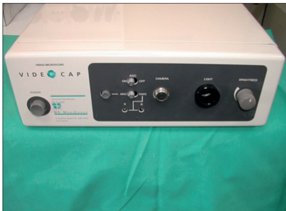
Figure 1. Central body, of videocapillaroscope, that includes a light source consisting of a cold halogen light emitted by a 100 W lamp fitted with an automatic or manual control device to regulate luminosity and white balancing.
