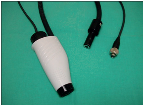
Figure 2. Probe with an optic terminal connected to the central body by a fibreoptic cable 2 metres in length; the optic terminal is in turn constituted by a colour high definition micro television camera (420.000 pixels), a support for holding the different lenses, a ferrule for fine focussing regulation, a radial ferrule at the tip with annular illumination (for a uniform illumination without shadows). The lenses which can be applied can be either contact or non-contact types with varying enlargements: 20×, 50×, 100×, 200×, 500×, 1000×.
