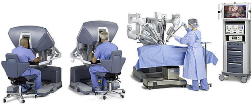
Fig. 1. The da Vinci robot surgical system consists of 1 or 2 surgical consoles, a patient cart, and a vision cart. (From Pietrabissa A, et al. Cirugía robótica: controversias actuales y expectativas futuras. Cir Esp. 2013;91:67–71.)
