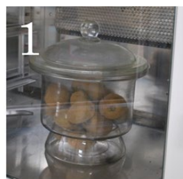
1 Exposing the fruits to 100 ppm of ethylene at 20°C for 24 h using sealed desiccator.
