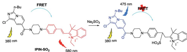
Scheme 2 Proposed sensing mechanism of IPIN-SO 2 with SO 3 2- .
