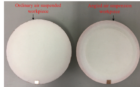
FIGURE 9: Ordinary suspension workpiece and suspended workpiece with angles of attack.
