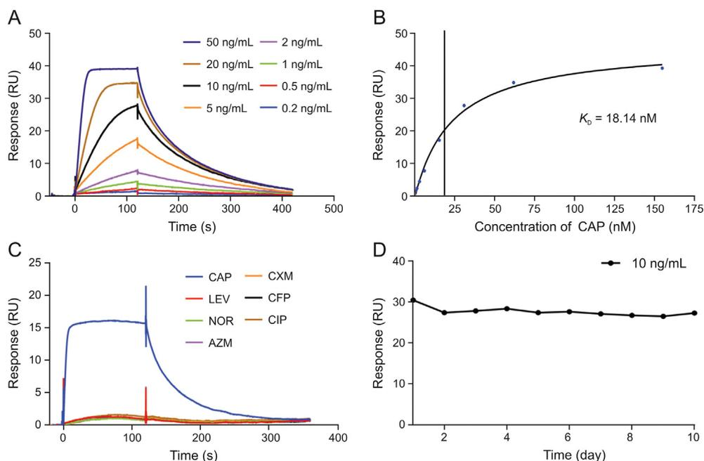
**Fig. 2.** Characterization of the surface plasmon resonance (SPR) sensor chip. (A) Sensorgrams of chloramphenicol (CAP) at different concentrations. (B) Fitting curves of CAP. (C) Response of CAP, ciprofloxacin (CIP), levofloxacin (LEV), norfloxacin (NOR), azithromycin (AZM), cefuroxime (CXM), and cefoperazone (CFP) with CAP antibody on CM5 chip. (D) Response of 10  $\text{ng}/\text{mL}$  CAP sample for 10 consecutive days.
