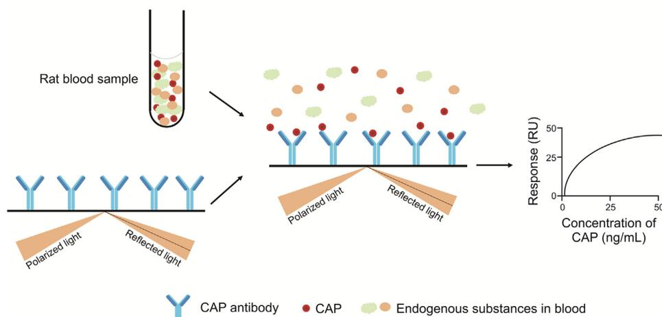
Fig. 1. Principle of the surface plasmon resonance (SPR) biosensor for the process of chloramphenicol (CAP) detection in rat blood samples.
