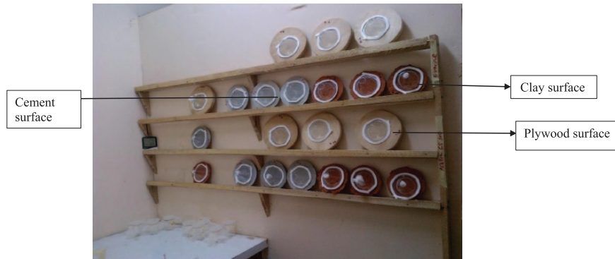
Figure 1. Cone bioassay test on different surfaces using deltamethrin at 0.02 g ai/m 2 and pirimiphos-methyl at 1 g ai/m 2 against Culex quinquefasciatus .
