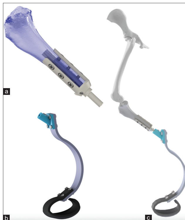
Figure-2: (a) A schematic of an osseointegrated transtibial hind-limb canine endo-prosthesis intramedullary implanted; (b) a schematic of an exo-prosthesis to be attached to the endo-prosthesis; (c) a schematic of the assembled hind-limb endo-exo-prosthesis.
