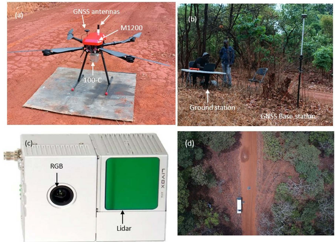
Fig 3. (a) T-Drone M1200 platform with 100-C sensor, (b) ground station and GNSS base station, (c) 100-sensor, and (d) aerial view of launch station.
