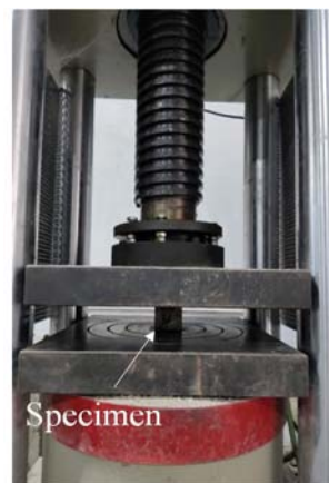
Figure 3. Diagram of compressive test.
