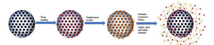
Figure 4. Schematic illustration of smart MSNs with the stimulus-responsive system.
