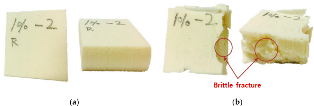
Figure 10. Fracture characteristics of PUF-silica aerogel (1 wt.%) composites owing to compression tests at (a) room (20 °C) temperature and (b) cryogenic temperature (−163 °C).
