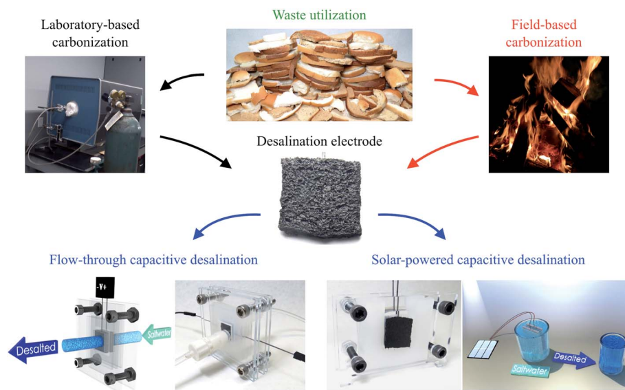
Fig. 1 Utilization of bread for water desalination. Conductive freestanding carbon electrodes were fabricated from bread using a common laboratory-based technique and a non-laboratory-based fire-based approach. Thermal treatment with both techniques yielded high surface area carbon electrodes which were then used for desalination in a capacitive deionization (CDI) system. The hierarchical pore structure of the freestanding bread electrodes enabled high salt adsorption and low resistance to water permeation in a flow-through (FT)-CDI system. Also, coupling the bread electrodes fabricated by fire with solar energy suggests a feasible solution to water desalination in economically burdened and remote regions.
