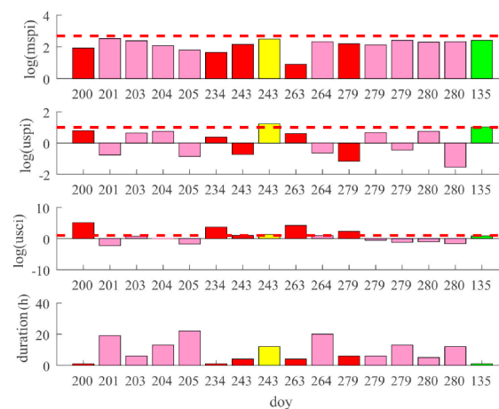
Figure 5. Unhealthy state statistics of C011. The subfigures correspond to m_{spi} , u_{spi} , u_{sci} , and duration of the unhealthy states, respectively. Green bars represent Type 2 unhealthy states. Red bars represent Type 3 unhealthy states. Yellow bars represent Type 4 unhealthy states. Pink bars represent Type 5 unhealthy states.
