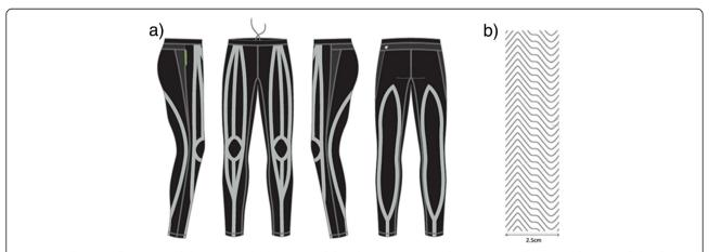
Figure 2 Schematic illustration of the CGSS with placement of the silicone stripes on the anterior and posterior leg (a) and detailed structure of the adhesive silicone stripes on the inner lining of the garment (b).
