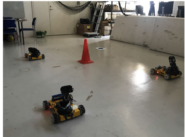
Fig. 1 The experimental setup demonstrating the proposed framework. Three Nexus 10011 mobile robots, in the workspace of Smart Mobility Lab (SML) (n.d.) that contains 5 RoI
