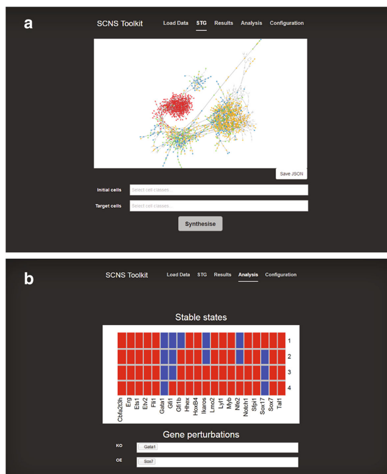
Fig. 1 Tool overview. When SCNS is first started, the user is presented with the ‘Load Data’ page, asking them to upload a .CSV file containing their single-cell gene expression data. a The state transition graph page, which allows visualisation of the data, selection of initial and target cell classes, and running of synthesis. b The analysis page, which shows the computed stable states of the synthesised model and allows combined overexpression/knockout perturbations to be run
