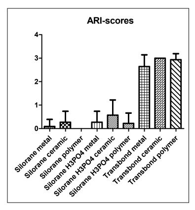
**Figure 2.** ARI scores of all test groups. High ARI scores indicate a fracture at the adhesive–enamel interface. Low scores indicate fractures between adhesive and bracket.
