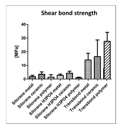
**Figure 1.** Mean shear bond strength and standard deviations. Significant differences ( $p \le 0.05$ ) were found between the Filtek Silorane and the Transbond XT groups.
