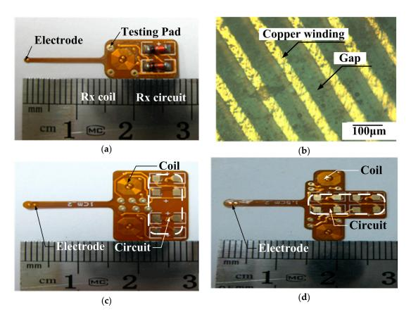
**Figure 5.** (a) Photograph of the single channel stimulator board; (b) Microscope image of the four-layer FPC coil (local). The four-layer FPC coils have a line width and spacing of 50  $\mu$ m and a thickness of 17.5  $\mu$ m; (c) A two-channel IPG interface with 10mm coils center distance; (d) A two-channel IPG interface with 15 mm coils center distance.
