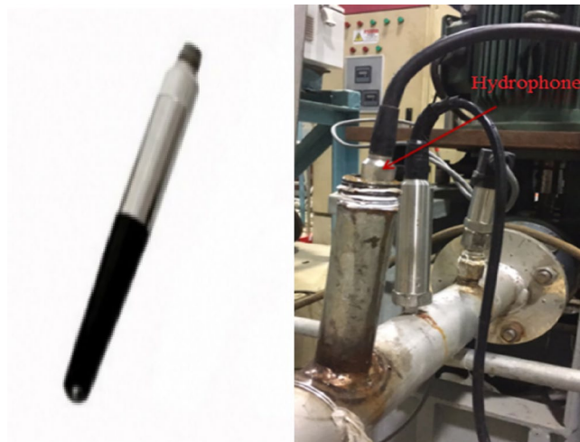
Figure 10. Hydrophone and installation location.
