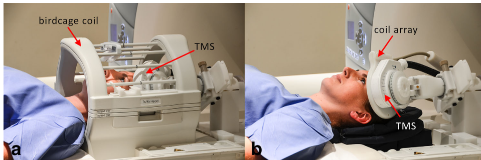
FIG. 1. (a) Conventional setup for concurrent TMS/fMRI experiments. The TMS coil is placed between the birdcage coil and the head of the subject. (b) New setup using the novel coil array. The MR coil array is placed between TMS and the head of the subject.
