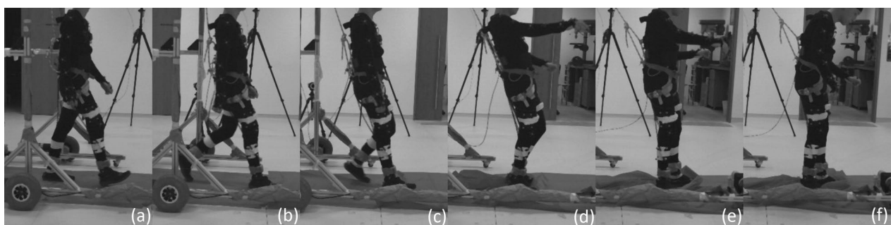
Fig. 15 Slip fall sequence (running from left to right) induced by the motor attached to the subject's ankle via the ankle cable wire rope. A low friction sliding sheet was placed on the ground to reduce the friction between the foot and the ground. Series of events: a ) left foot approaching the end of swing phase; b ) left foot enters the stance phase and perturbation is applied (motor starts pulling); c ) perturbed left foot slides forward and the right legs straightens for touchdown; d ) right foot touches down and slide forward together with the left foot; e ) both legs slide forward together; f ) sliding stops and subject is recovering to a standing posture
