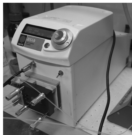
Figure 21. The commercially available Syrris Asia electrocatalytic reactor system.
