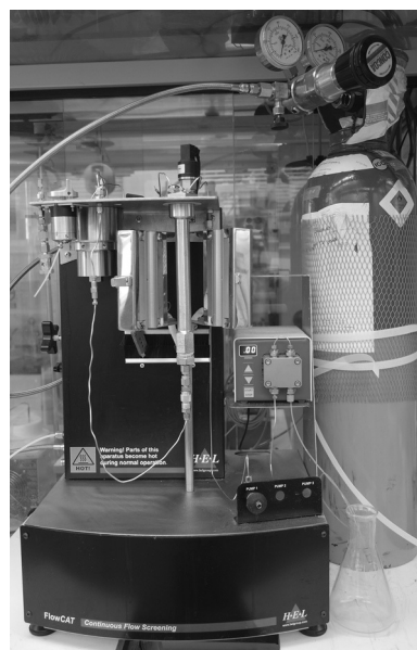
Figure 8. The HEL FlowCAT trickle-flow reactor has been used for the hydrogenation of ethyl nicotinate over a packed-bed catalyst.
