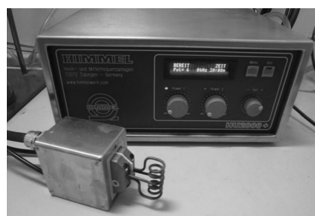
Figure 11. An inductive system used for the machine-assisted heating of a continuous-flow reactor column. Reprinted from Ref. [54a].
