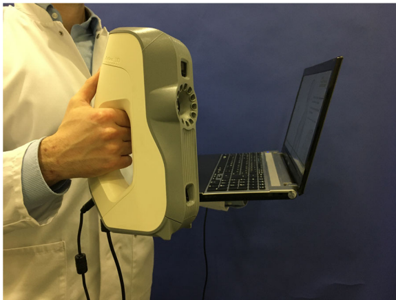
Fig. 1 The mobile structured-light surface scanner Artec Eva (Artec 3D Inc., Luxembourg) used for all imaging procedures
