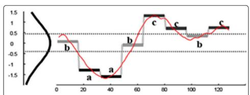
**Figure 2** A real valued time-series can be converted to the SAX word baabccbc. The y-axis represents z-scores. *Note.* Adapted with permission from "Assumption-Free Anomaly Detection in Time Series," by Wei et al. [11].
