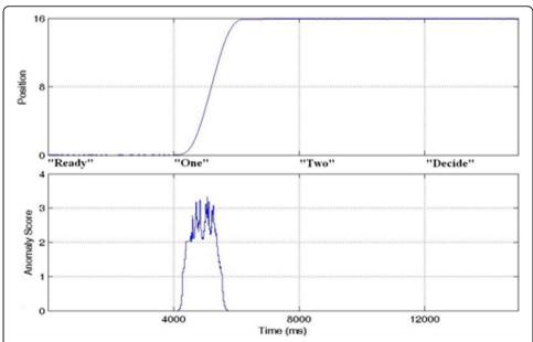
**Figure 4 Time series record of the platform position (a) and anomaly score (b).** Both signals indicate where actual movement has occurred. The dotted lines in this and subsequent figures denote the four test intervals.
