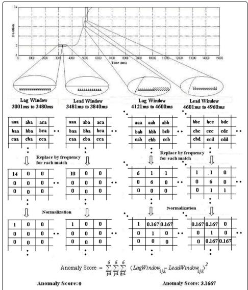
**Figure 3 Method illustrating Time-Series-Bitmap Algorithm**. Illustrating conversion of data subsequences into SAX symbols to calculate anomaly scores for each instance of the lag and the lead windows using the known time-series data of platform position taken from a move in Interval 1. *Note*. Adapted with permission from Bhatkar et al, 2006 [19].
