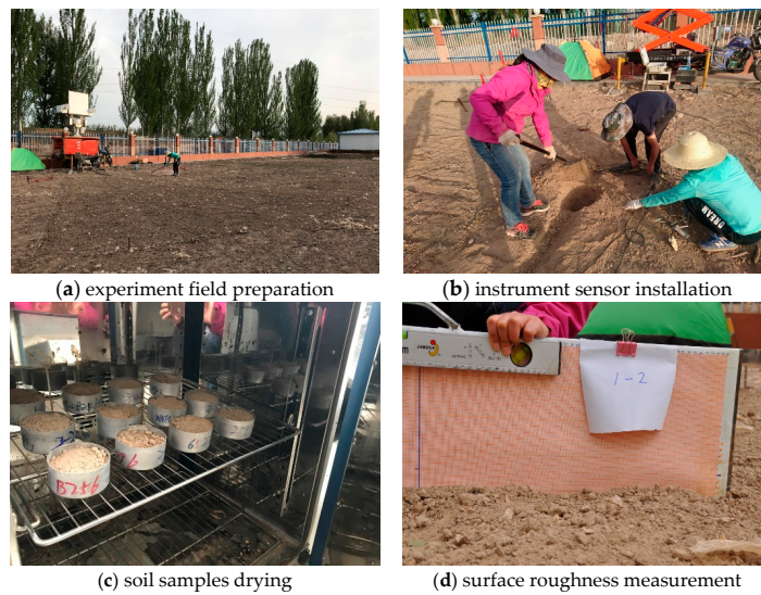
Figure 1. The observation experiment of soil moisture and soil salinity.
