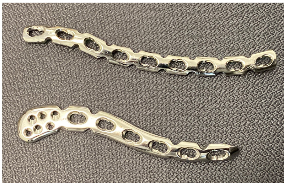
Fig. 2 A reconstruction locking plate (above) and anatomic locking compression plate (below) removed from two patients with right-sided clavicle fractures
