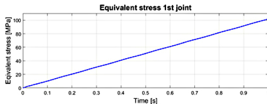
Figure 22. The course of stress reduced according to the von Mises hypothesis during the analysis of transient states—movement in the first joint of surgical robot.
