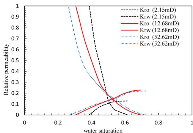
**Figure 2.** Janus smart nanocapsule dispersion system/oil relative permeability curve.
