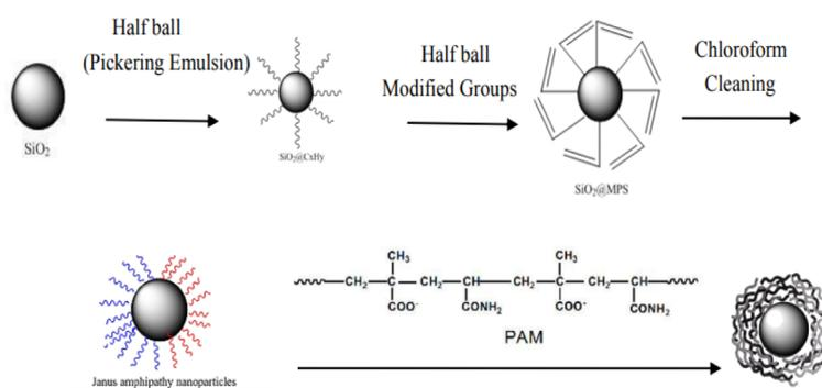
**Figure 1.** Synthetic route and action diagram of Janus nano oil displacement agent. (a) Schematic diagram of small-size crude oil formed after the action of Janus nanoparticles. (b) Synthesis route of the Janus nanocapsule.
