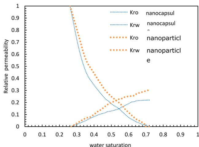
**Figure 5.** Comparison of Janus intelligent nanocapsule dispersion system (52.62 mD) and Janus functional particle (50.78 mD) oil relative permeability curve.
