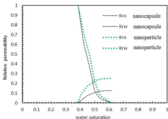
**Figure 3.** Comparison of Janus intelligent nanocapsule dispersion system (2.15 mD) and Janus functional particle (2.57 mD) oil relative permeability curve.
