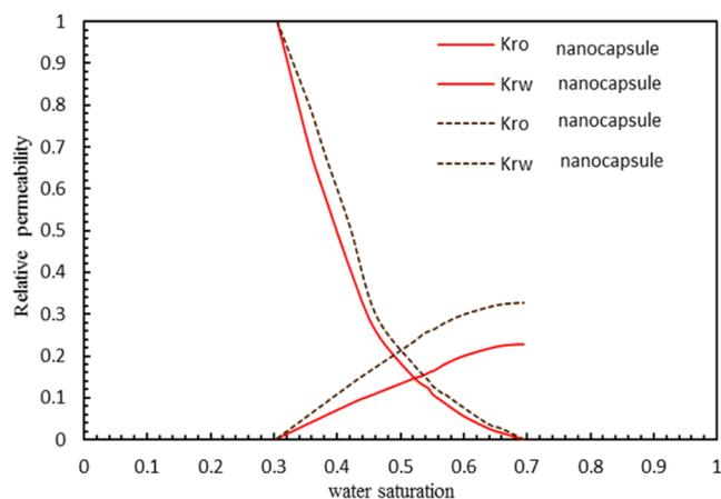
**Figure 4.** Comparison of Janus intelligent nanocapsule dispersion system (12.68 mD) and Janus functional particle (12.68 mD) oil relative permeability curve.
