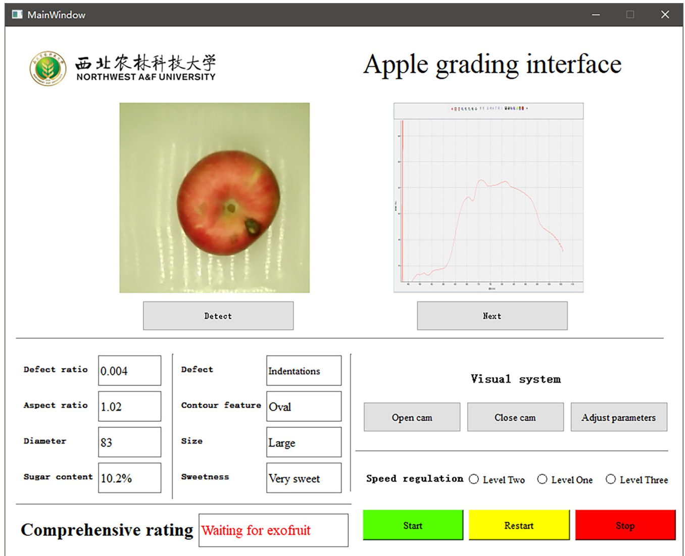
Fig 17. The interface of the apple quality grading software.
